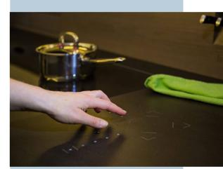
Fingertip finesse: The Touch Surface from Loxone can transform surfaces into a capacitive touch switch for the control of lighting, blinds and multi-room audio – only activating when needed. It can work on stone, wood, ceramic or glass surfaces. It can be battery or permanently powered, Loxone says.
